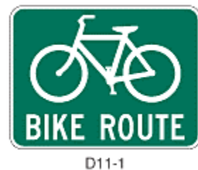
Figure 3.6. Typical Bike Route sign. Source: MUTCD.
