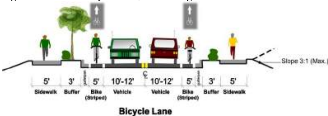
Figure 4.5. Marked Bicycle Lane, No Parking*
